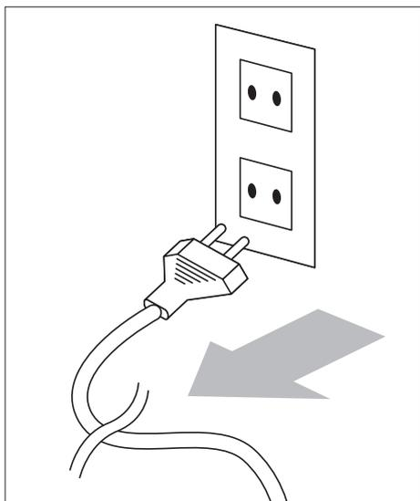
The power can be turned off immediately in an emergency by removing the plug from the power outlet. Make sure that there are no obstructions around the power outlet when using this equipment.
