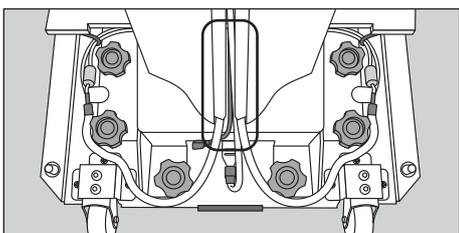
Insert the cables from both grips into the slit on the column.
