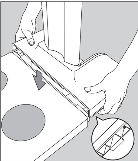
Fit into place and lock the cover to the platform.
