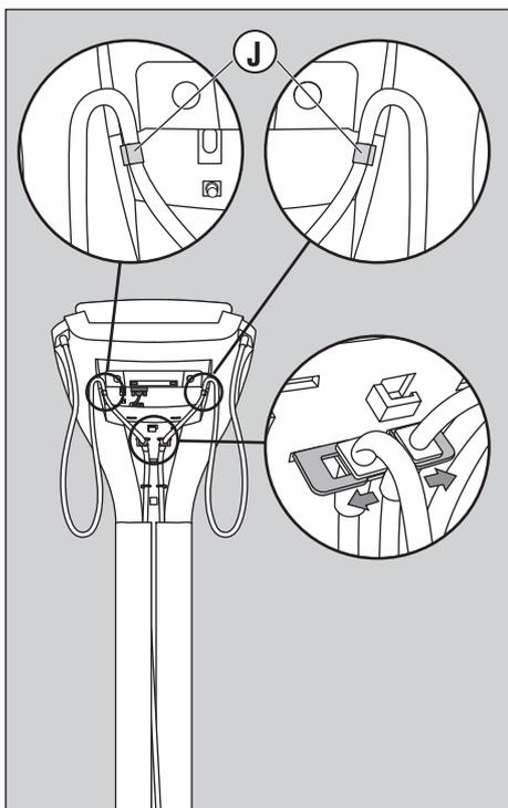
Fix the cables from both grips to the column using clamp **J** as shown in the figure on the left.
