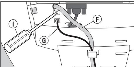
Fix these two cables into place with the hook at the top of the column. Insert the plugs for the power supply cord and the communication cable to the respective connector on the display unit. Use the provided screwdriver (I) to fix the communication connector firmly into place.
