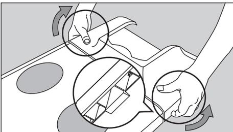
Pull the two tabs at the right end and the left end of the cover (large) toward the outside and remove the cover.
